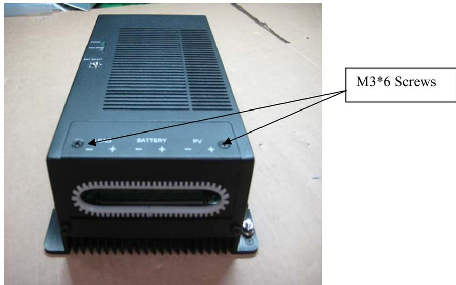
Remove these screws M3\*6 (\*2) from the top cover to access the terminal blocks of controller
